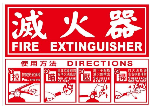
Fire Extinguisher Directions
